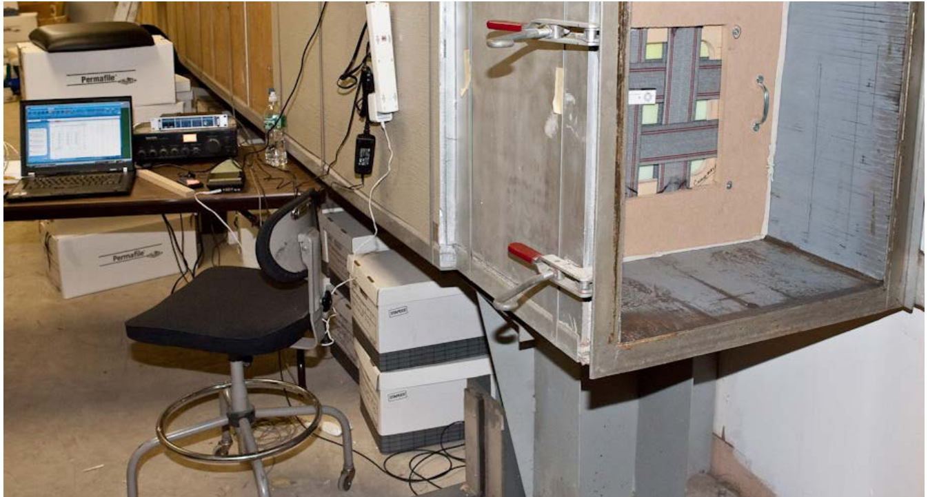
Impedance tube loaded with sample seat bottom for acoustical measurement
