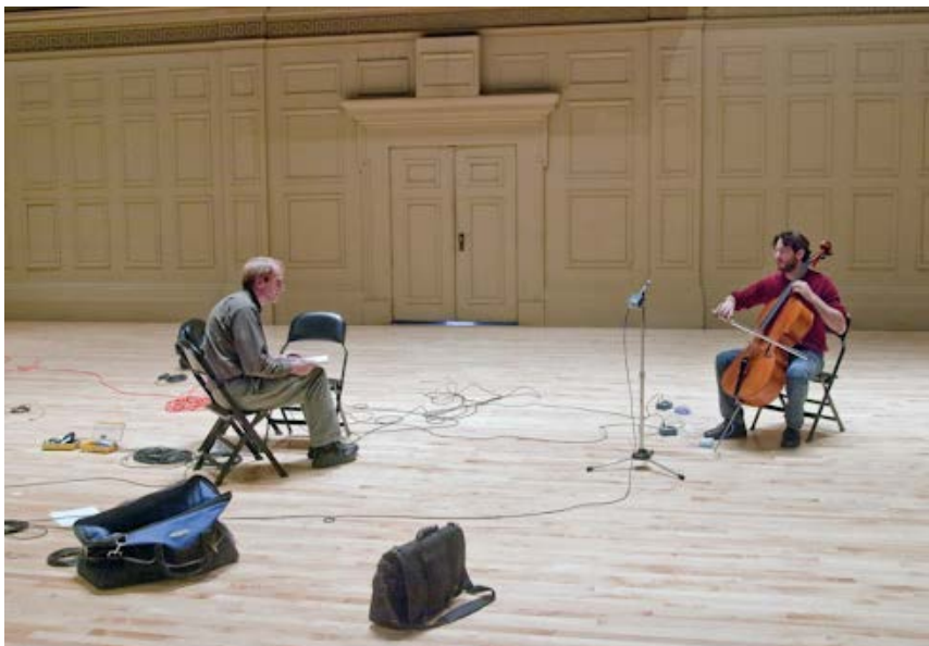
Acousticians James Moore and Jonah Sacks measure the response of the new stage floor to excitation by cello.
