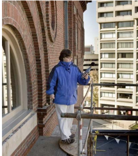
Measuring sound levels on the roof outside concert hall clerestory windows
