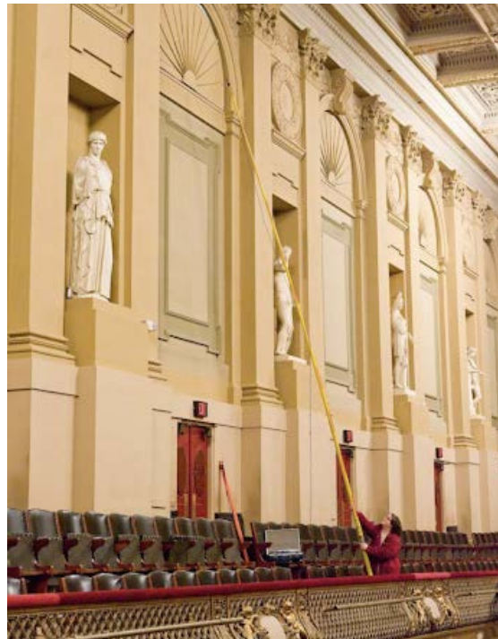
Measuring sound transmission through a shuttered clerestory window in the concert hall
